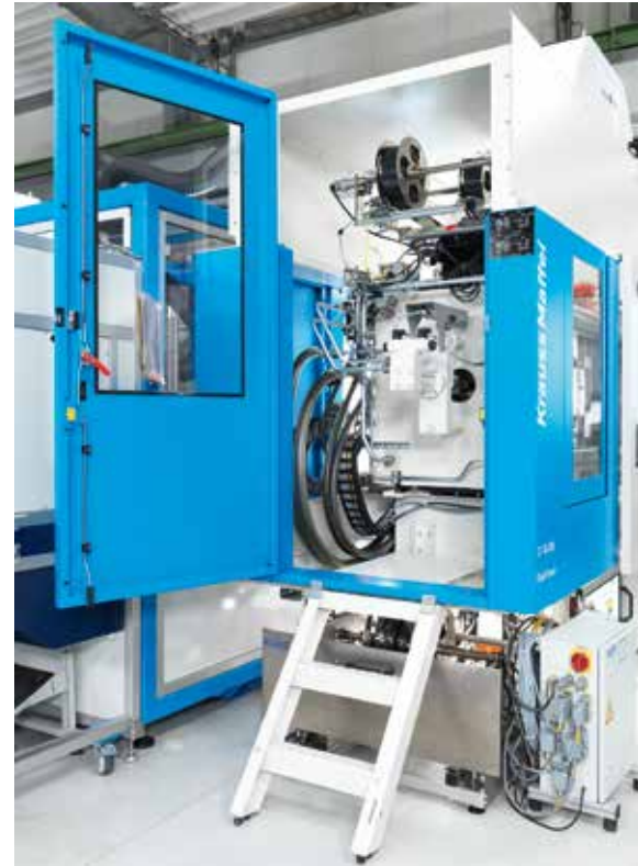
Fig. 6. The two-platen machines of the CX series make very efficient use of the installation area for the IMD process and ensure outstanding accessibility of all components thanks to their ejector space door (© KraussMaffei)
