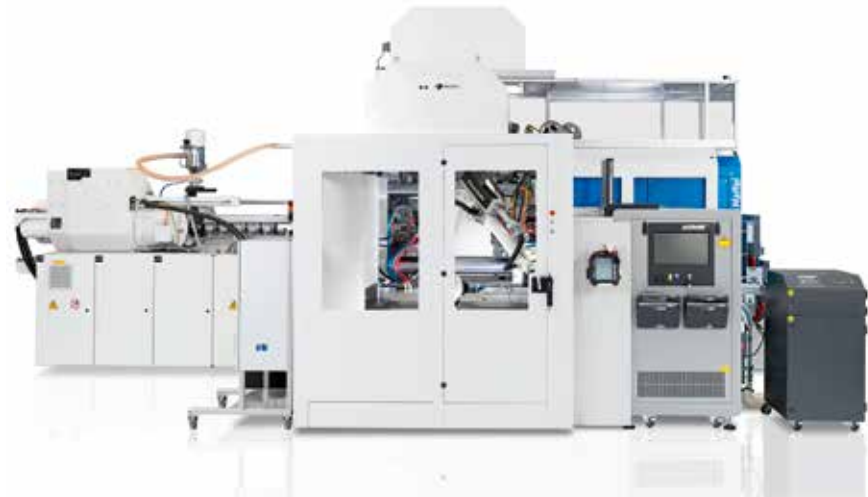
Fig. 1. Compact and flexible at the same time: the all-electric PX 320 with integrated automation cell combines the IMD and IML processes (© KraussMaffei)
