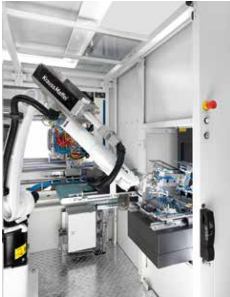
Fig. 5. Compact automation: a six-axis robot inserts the components into the laser trimming station. Visible in the background: the conveyor with UV tunnel and, behind it, the clamping unit with the film feed (© KraussMaffei)
